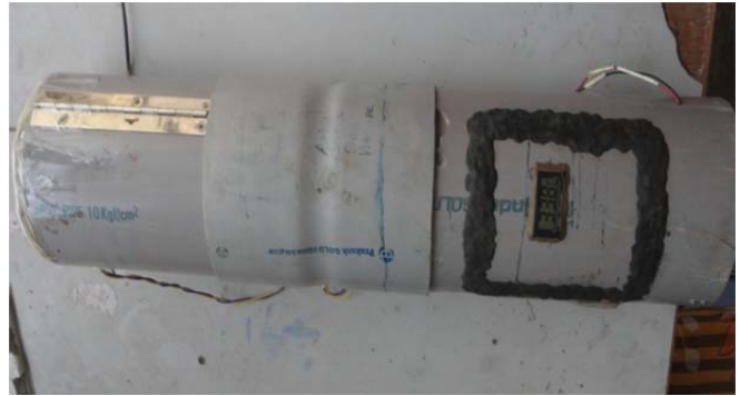
Fig. 8 Complete final assembly of Thermoacoustic Refrigerator
